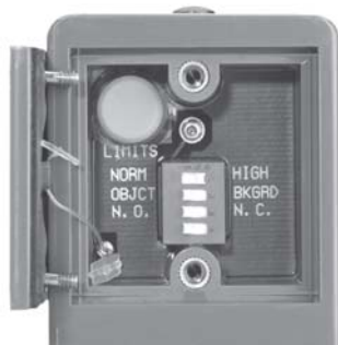
SM500 Control Compartment with Sealed Door
